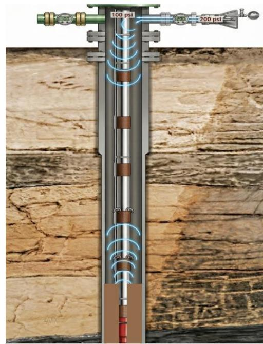
A chamber that measures the volume of air volume flowing into the annulus in response to the displaced mud
